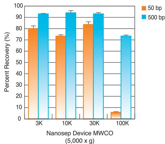
A 500  $\mu\text{L}$  sample of a 100  $\mu\text{g}/\text{mL}$  DNA fragment solution containing 50 and 500 bp double-stranded DNA fragments was centrifuged at 5,000  $\times g$  in Nanosep devices to a final volume of 50  $\mu\text{L}$ . Recovered samples were quantified using absorbance at 260 nm. The 100K device was able to differentiate between the sizes of the DNA fragments.
