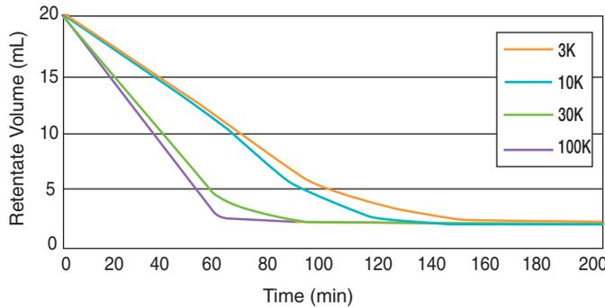
Protein solutions were processed in each of the Macrosep Advance devices. Average time (minutes) is plotted against mL of remaining product to be filtered using a swinging bucket rotor at 5,000 x g. Solutions are 3K: Protamine Sulfate, 0.1% in 1X PBS; 10K: Cytochrome C, 0.025% in 1X PBS; 30K: IgG, 0.1% in 1X PBS; and 100K: Apoferritin, 0.1% in 1X PBS.
