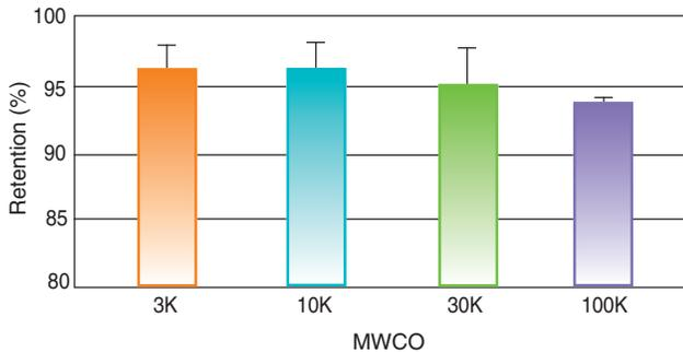
Protein solutions were processed in each of the Macrosep Advance devices. Average percent retention using a swinging bucket rotor at 5,000 x g is displayed for each MWCO. Solutions were 3K: Protamine Sulfate, 0.1% 1X PBS; 10K: Cytochrome C, 0.025% in 1X PBS; 30K: IgG, 0.1% in 1X PBS; and 100K: Apoferritin, 0.1% in 1X PBS.
