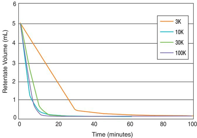
Protein solutions were processed in each of the Microsep Advance devices. Average time (minutes) is plotted against mL of remaining product to be filtered using a 34° fixed angle rotor at 5,000 g. Solutions are 3K: Cytochrome C, 250 µg/mL; 10K: BSA, 1 mg/mL; 30K: IgG, 1 mg/mL; and 100K: Thyroglobulin, 1 mg/mL.
